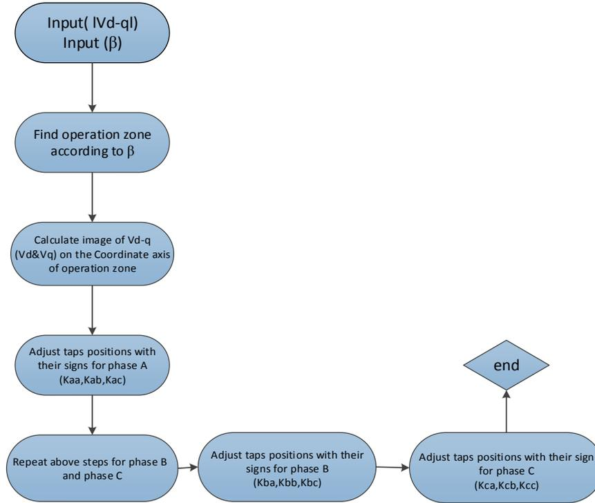
Figure 7. Flow chart for matlab codes to determine taps position
