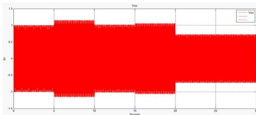
Figure 11. Changes in value of sending end voltage (Vse)
