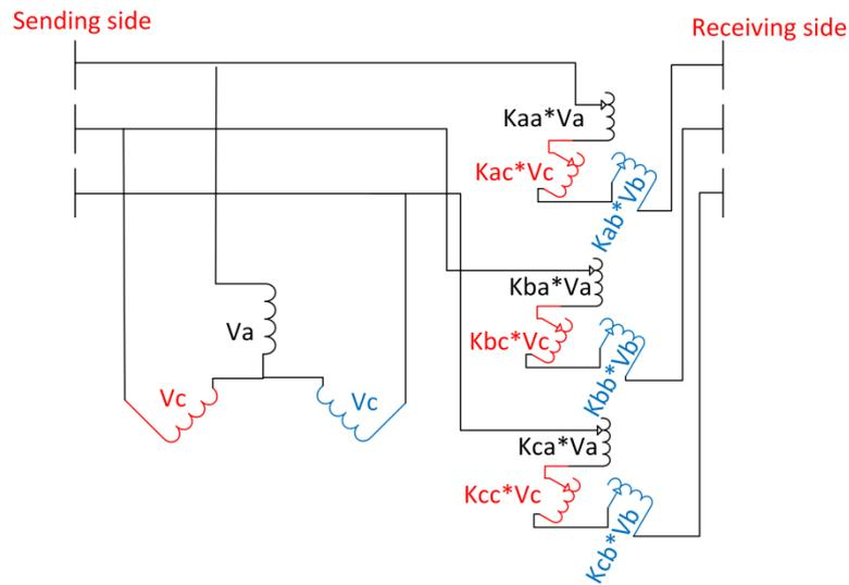
Figure 3. Schematic diagram of conventional ST
