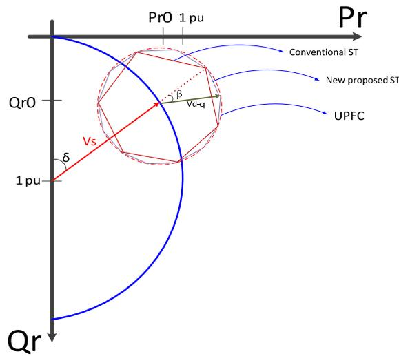
Figure 9. Relationship between Pr and Qr In the presence of UPFC, conventional ST and new expressed ST
