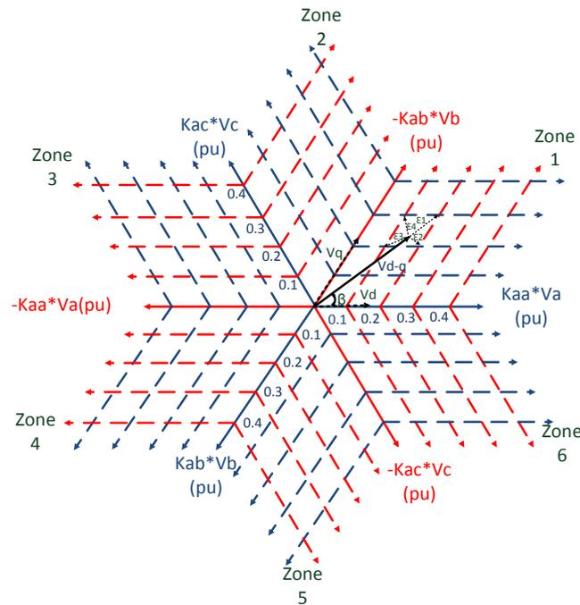
Figure 6. Tap position grid for the construction of  $V_{d-q}$
