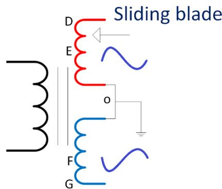
Figure 4. Three winding linear transformer
