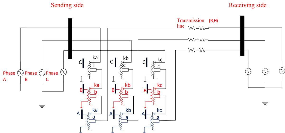
Figure 5. General structure of transmission line and ST windings
