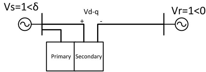
Figure 1. Location of Sen Transformer in transmission line
